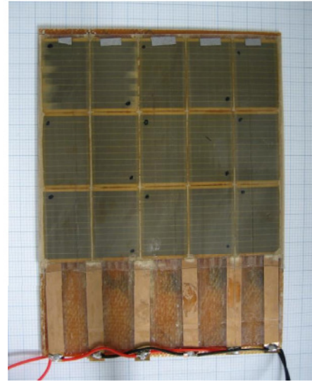
Fig. 11 : Array of piezoceramic stacks for multi-morph bending actuator
