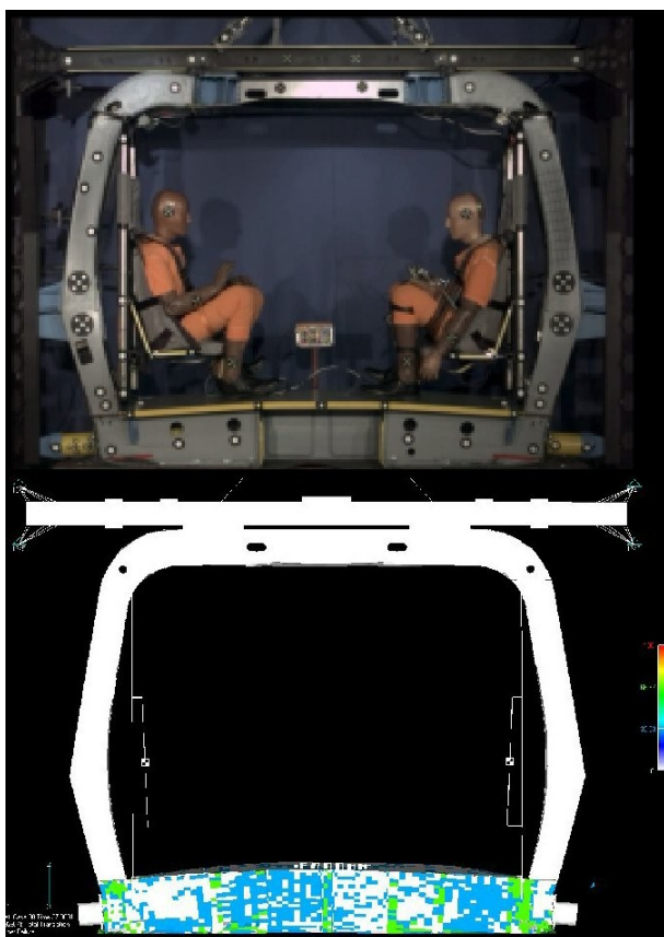
Figure 4: NH90 Fuselage Section, Drop-Test and Simulation
