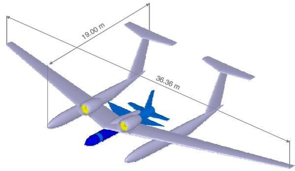
FIG 17. UAV system with the space launcher
