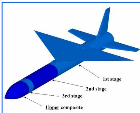
FIG 13. Baseline launcher configuration
