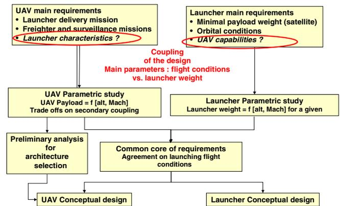
FIG 15. Joint UAV/launcher design methodology
