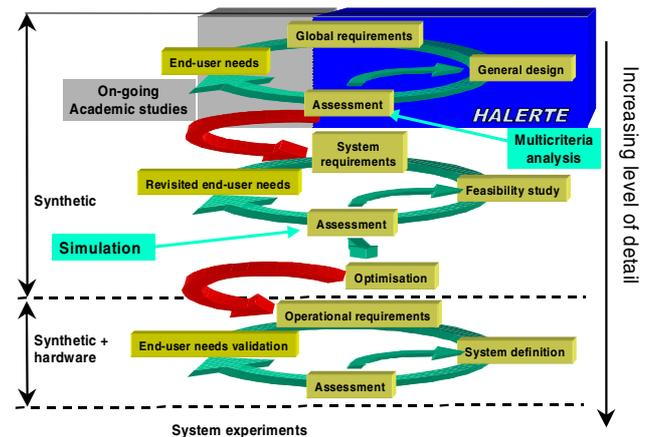
FIG 4. Overall design process
