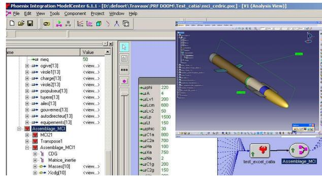
FIG 21. Integration of a CAD model in ModelCenter
