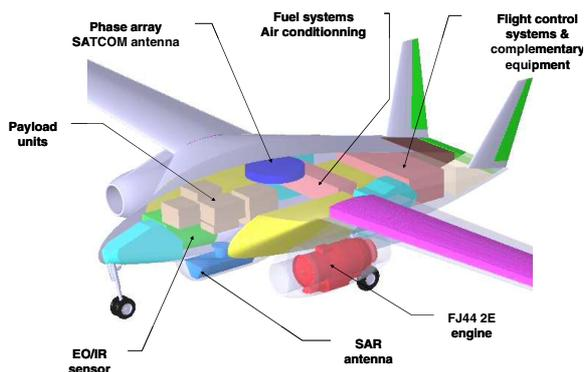
FIG 12. Internal view of OBW-02 configuration
