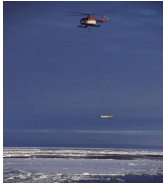
Fig. 2 Ice Thickness Measurement with AWI EM-Bird
