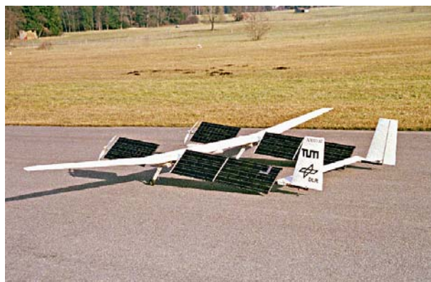
Figure 4 Solitair-1 solar powered remotely controlled aircraft on the DLR Braunschweig airfield
