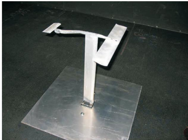
Figure 1: The DLR F13 model in wind tunnel facility C at TUM-AER
