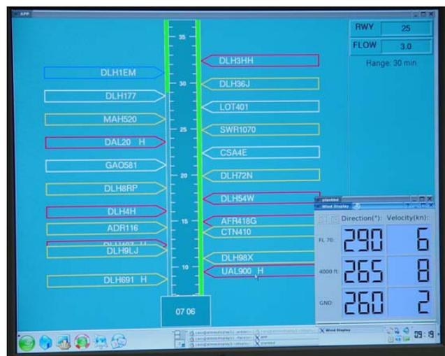
FIG 10. Controller's planning screen with dynamic time scale and wind information.
