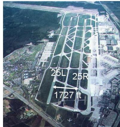
FIG 1. Frankfurt Airport with the two parallel runways 25L and 25R, spaced by 1727 feet (518 m).
