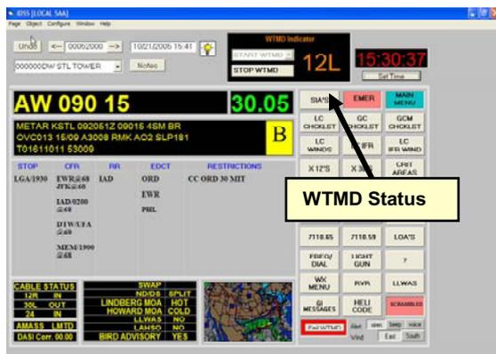
FIG 8. Overview of ACE-IDS Display With WTMD Status Field
