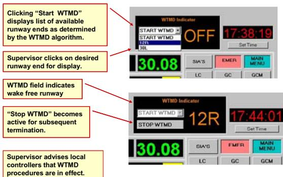
FIG 9. WTMD Display Supervisor Controls
