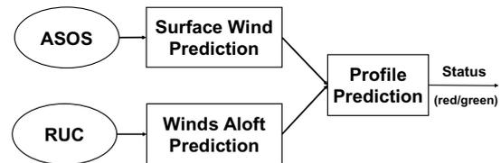
FIG 4. Block Diagram of Wind Forecast Algorithm Functional Logic
