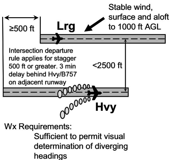
FIG 2. WTMD Wind Conditions
