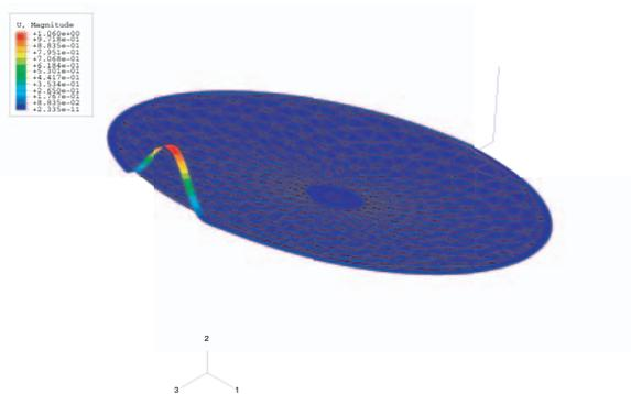
FIG. 7: First Buckling Mode of SSBR.
