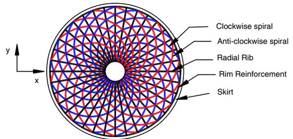
FIG. 3: Configuration of the Full-Scale SSBR.
