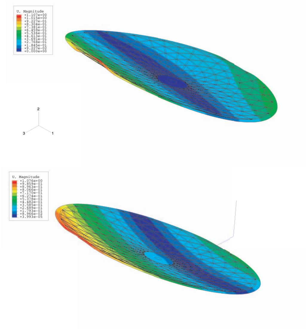
FIG. 6: Mode 1: (a) SSBR on a Rigid Interface, top, (b) SSBR attached to the boom, bottom
