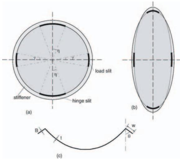
FIG. 2: Adjustable Parameters of the Stiffening System.
