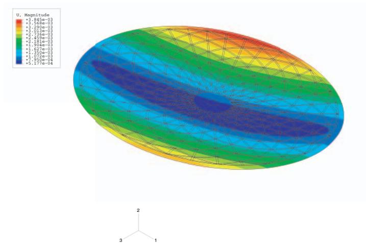
FIG. 5: Displacement Magnitudes due to Thermal Loading.
