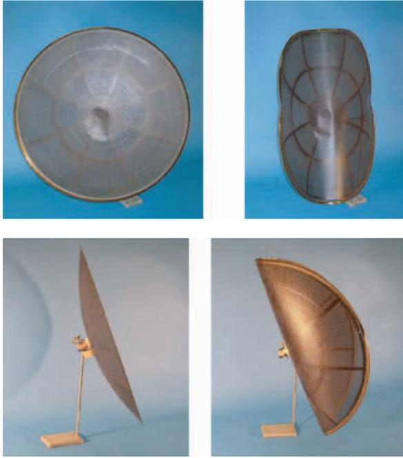
FIG. 1: Stiffened Spring Back Reflector Demonstrator.
