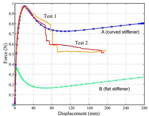
FIG. 9: Packaging Behaviour of Experimental and Finite Element Simulations for the 0.8m Demonstrator.
