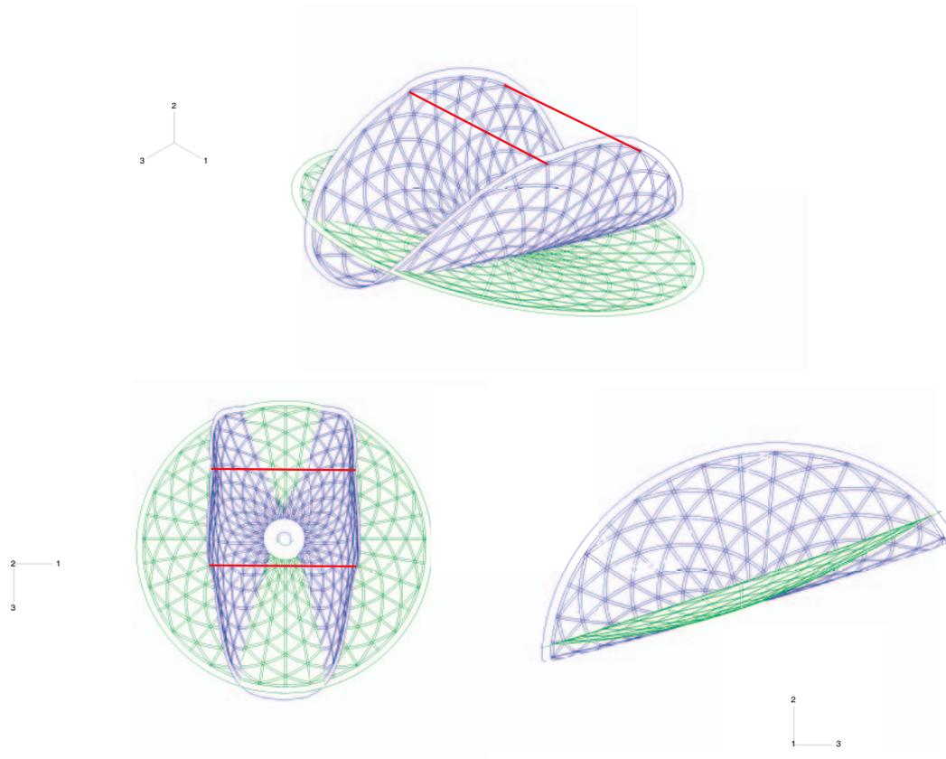
FIG. 8: SSBR in Deployed (Green) and Folded (Blue) Configurations; Tie Cables (Red).
