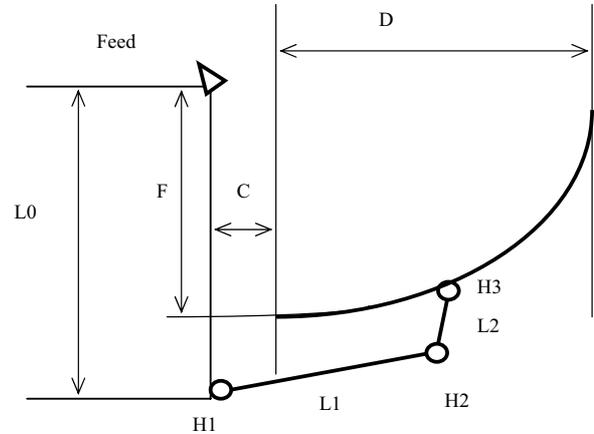
FIG. 4: Basic Definitions of the Boom Attachment.
