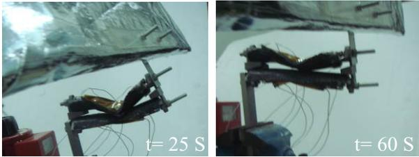
Fig.13 Process of deployment in a sequence of a prototype of a solar arrays actuated by SMPC hinge
