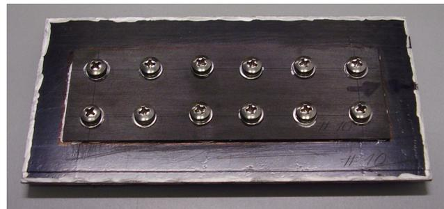
FIG. 2 Bolted joint shielding efficiency test sample
