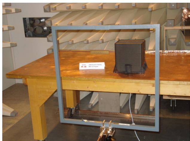
FIG. 13 CFRP electronic housing in the test chamber
