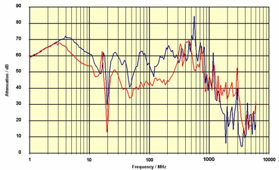
Electromagnetic shielding of SUMER DPU case (aluminium, +z axis irradiation)
