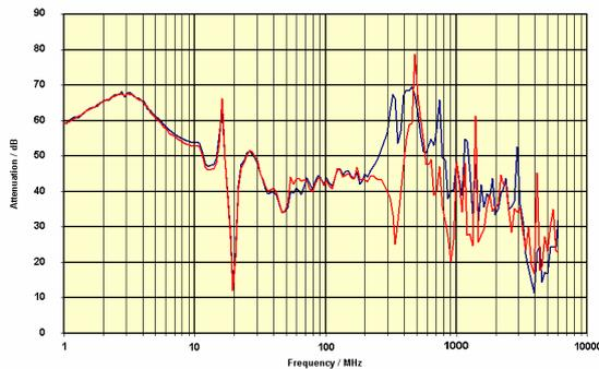
Electromagnetic shielding of CFRP case (+z axis irradiation, copper plated edges)
