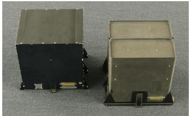
FIG. 5 The CFRP (right) and the AL reference electronic box
