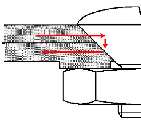
FIG. 10 Current path from bottom CFRP lid to CFRP flange via countersunk bolted joint (CFRP lid and flange are shown shaded.)
