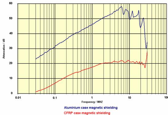
FIG. 14 Magnetic shielding efficiency of the aluminium and the CFRP case
