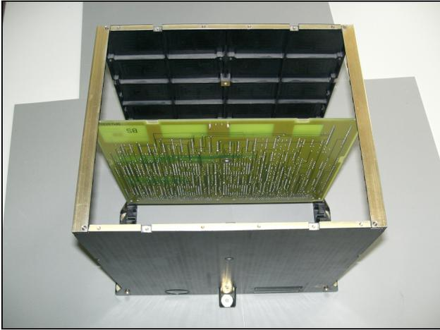
FIG. 6 SUMER DPU electronic housing, sheet metal panels removed
