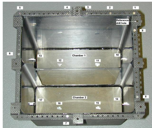
FIG. 11 View inside the CFRP case with points of bonding measurements
