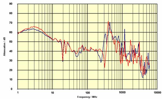
Electromagnetic shielding of CFRP case (+z axis irradiation, untreated edges)
