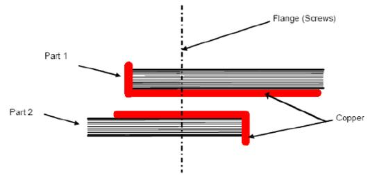
FIG. 4 Electrically seal bolted joint
