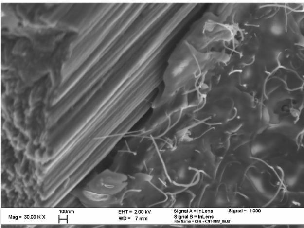
FIG. 3 Electron microscopic photo of a carbon fibre (left side) and a CNT modified epoxy matrix
