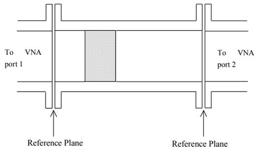
FIG. 1 Waveguide measurement of shielding efficiency. The test sample is shown hatched.
