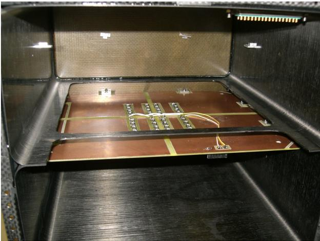
FIG. 9 Dummy PCB fixed with brackets in the CFRP housing. The centre wall between the cells was partly removed to create an electrically identical cavity as in the reference housing. The nickel coated carbon fibre mat is visible on the top cover of the housing.
