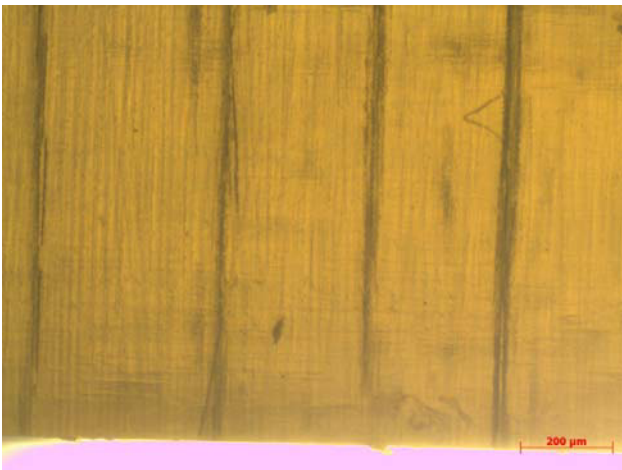
FIG 18. Multiple IFF cracks after higher loading (top view, 50 times magnification)
