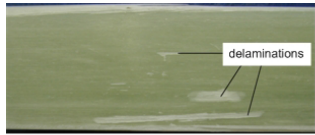
FIG 24. 0°-specimen after 100 000 cycles and a stiffness loss of 2.24 %
