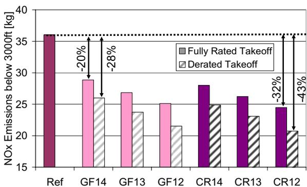
FIG 17. Low altitude NO<sub>x</sub>-Emissions (<3000ft)
