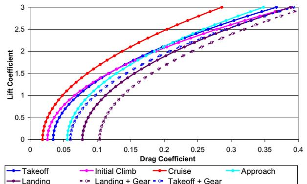
FIG 3. Aircraft drag polars<sup>1</sup>
