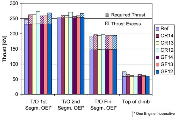
FIG 6. Thrust requirements
