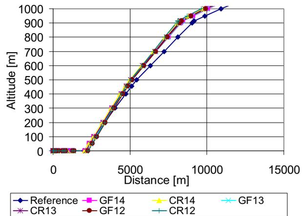
FIG 15. Low level takeoff-trajectory
