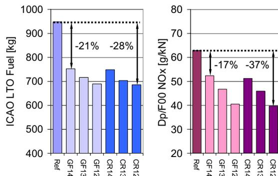
FIG 9. ICAO LTO fuel consumption and NO<sub>x</sub> emissions
