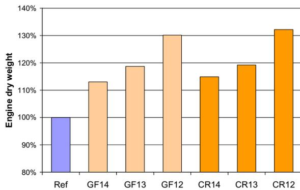
FIG 4. Engine dry weight relative to reference engine
