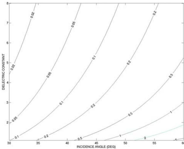
FIG 11. Relation between incidence angle, dielectric constant and echo power ratio<sup>(15)</sup>
