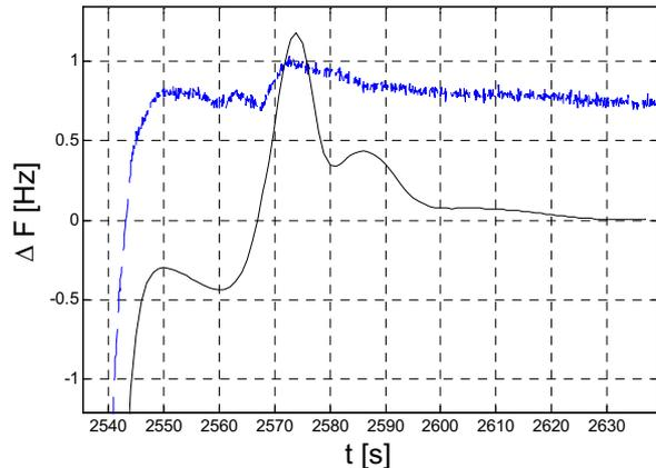
FIG 9. Comparison between the frequency shifts caused by ray bending in the planetary atmosphere and ionosphere of Venus. The dark line shows the predicted signal while the measurements are indicated in blue<sup>(13)</sup>
