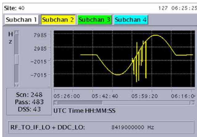
FIG 16. Results of OL recording at DSS 43, Canberra, Australia. Only atmospheric/ionospheric media contributions to the total frequency shift remain. Occultation pass in VEX orbit #381.
