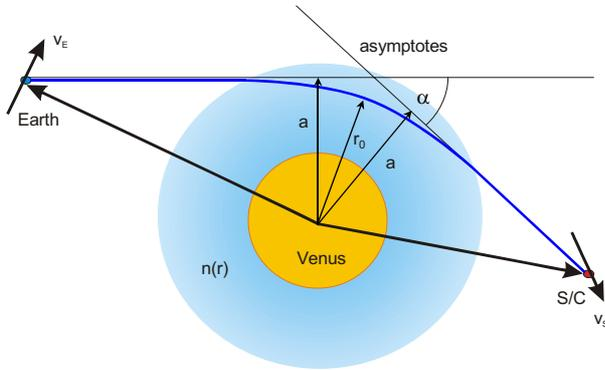
FIG 6. Ray bending in the Venus atmosphere. Ray path closest approach distance  $r_o$  and deflection angle  $\alpha$  are related to the impact parameters  $a$  (asymptote closest approach distance) and index of refraction  $n(r)$ . The  $(x,z)$  coordinate system is a planetocentric coordinate system. <sup>(1)</sup>
