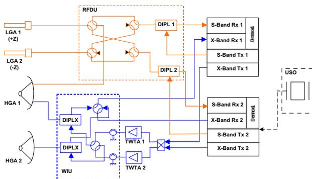
FIG 1. Block diagram of the S/C communication subsystem (courtesy EADS-ASTRIUM)
