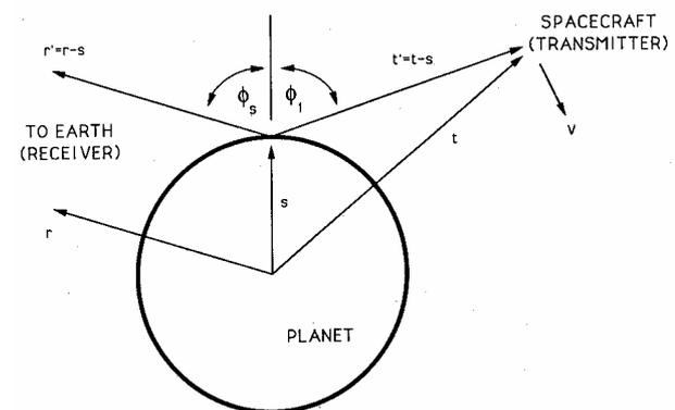
FIG 10. Geometry for the Bistatic Radar Experiment<sup>(14)</sup>
