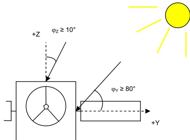
FIG 13. VEX S/C sun illumination - thermal constraints
