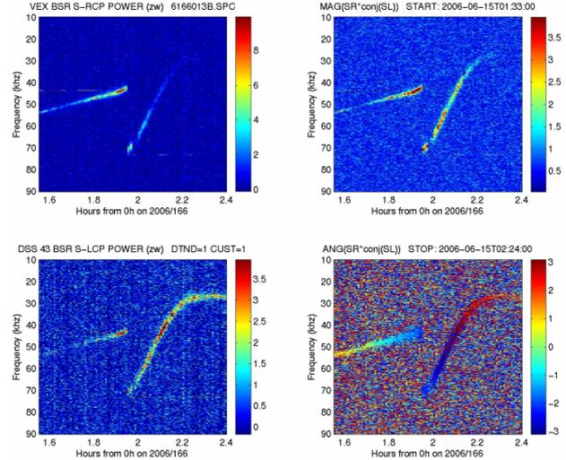
FIG 12. Echo signals from Venus surface during a BSR experiment over Maxwell Montes: frequency spectrum of right and left circular polarization (left side) and cross spectrum (magnitude and phase, right side)<sup>(15)</sup>.
