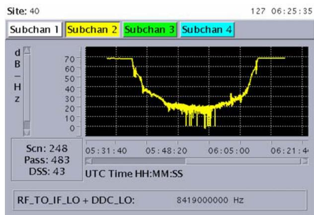
FIG 17. Results of OL recording at NASA DSS 43, Canberra, Australia. Received RF carrier power (spectral power density) vs. time. VEX occultation pass, orbit #381.
