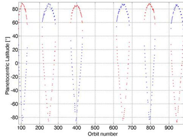
FIG 5. Distribution of planetocentric latitudes for occultation ingress and egress (assumed to be at the planetary surface) for nominal and extended mission (red dots mark occultation ingress, blue dots mark occultation egress) <sup>(1)</sup>.
