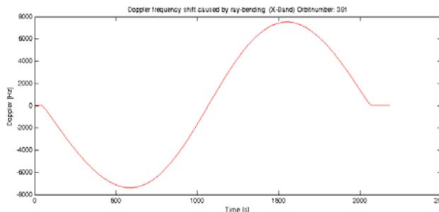
FIG 18. RSS predicted frequency shift caused by the atmospheric/ionospheric media for the same pass shown in fig. 17.
