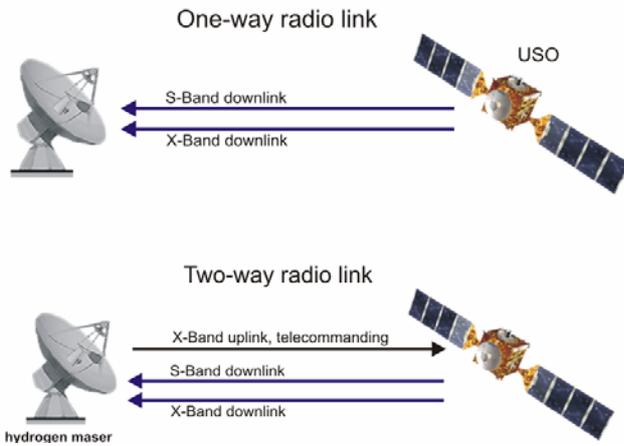
FIG 3. Transponder configurations and transmission modes of the satellite. The Ultra-Stable Oscillator (USO) serves as onboard reference frequency source in the One-Way mode. In the Two-Way mode the reference frequency is generated by a  $H_2$  – Maser.
