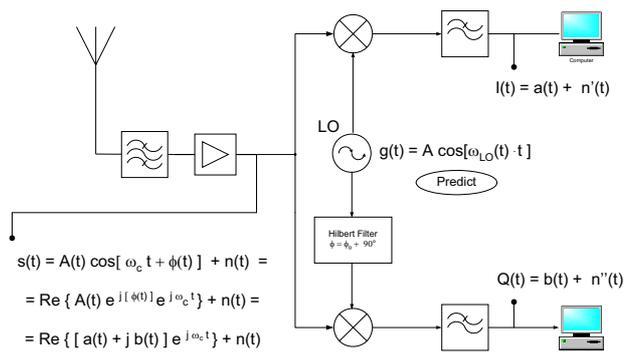
FIG 15. Principle scheme of a coherent receiver. The analogue base band components are extracted from the signal and stored separately.
