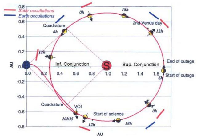
FIG 4. Venus position and observation geometry throughout the mission in a Sun-Earth fixed coordinate system.
