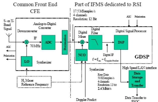
FIG 14. Principle scheme of the New Norcia IFMS Open Loop receiver <sup>(18)</sup>.
