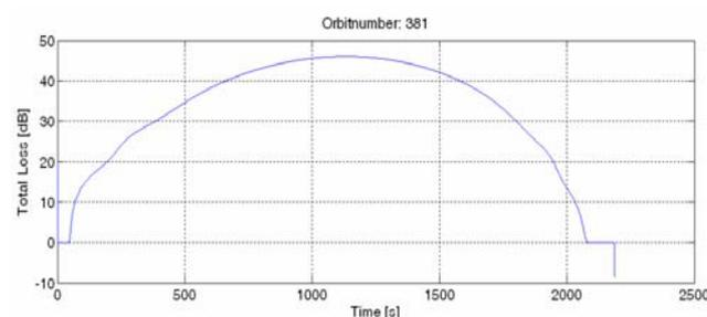
FIG 19. By the RSS predicted RF carrier power spectral density vs. time for the pass shown in fig. 18.
