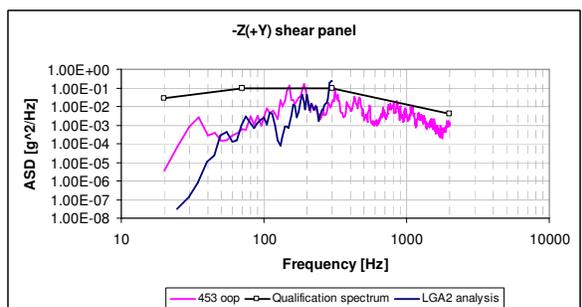
FIG 7.0-1d Test vs Random Vibration Analysis Results comparison (-Z+Y shear panel)
