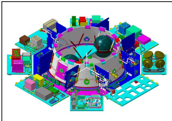
FIG 3.0-2 HERSCHEL internal configuration
