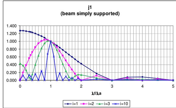
FIG 4.0-1 One-dimensional joint acceptance for simply supported beams
