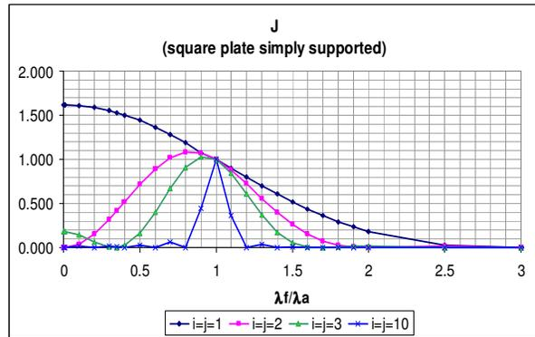
FIG 2.1-2 Two-dimensional joint acceptance for simply supported square plates
