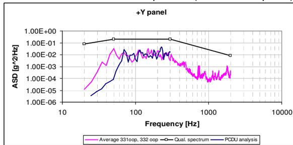
FIG 7.0-1b Test vs Random Vibration Analysis Results comparison (+Y lateral panel)
