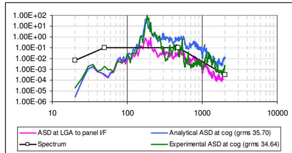
FIG 6.3-2 LGA tuned 1 d.o.f. transmissibility function validation
