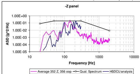
FIG 7.0-1c Test vs Random Vibration Analysis Results comparison (-Z lateral panel)
