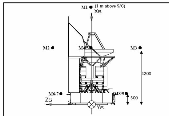
FIG 5.0-1a Acoustic test configuration
