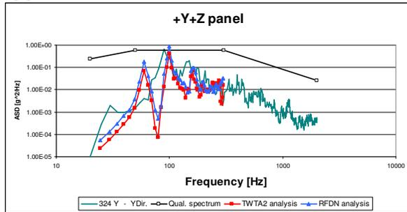
FIG 7.0-1a Test vs Random Vibration Analysis Results comparison (+Y+Z lateral panel)
