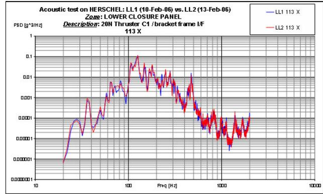
FIG 6.2-1 Pre- and post-low level runs comparison (20 N thruster)
