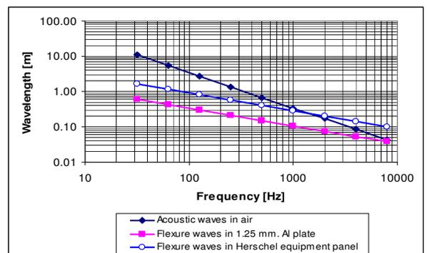
FIG 4.3-1 Acoustical and structural flexure wavelengths versus frequency
