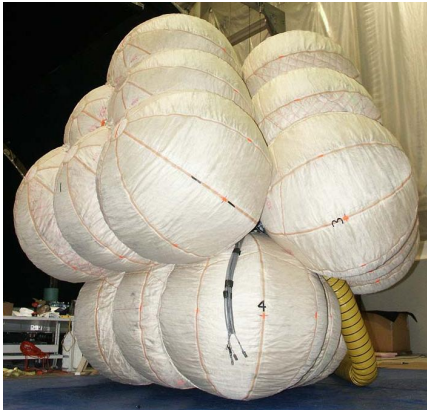
FIG 4. NASA Mars Exploration Rover landing airbags (NASA photo).
