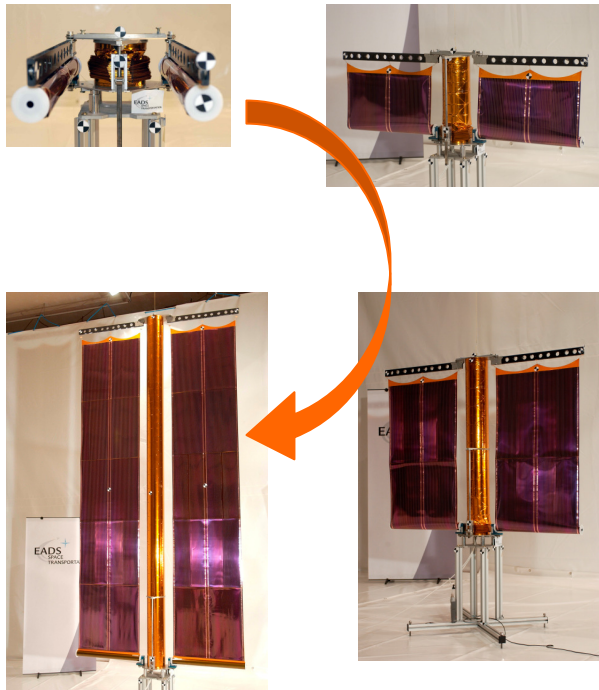
FIG.1 : Gossamer structure deployment concept
