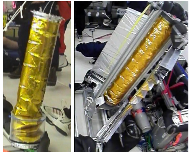
FIG.14 : 1 meter boom & 2 membranes breadboards
