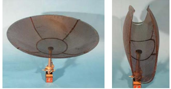
FIG. 2: Small scale model of the Stiffened Spring Back Reflector in deployed and packaged configuration
