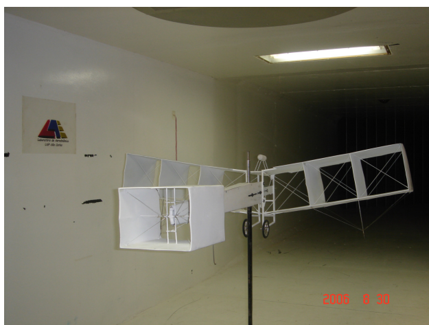
FIG 16 14-Bis model inside the wind tunnel.
