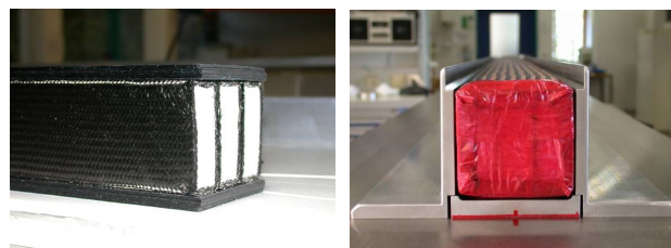
Fig. 6: Manufacture of the spar with prepreg cap belts (left); spar with final wrapping in the tool (right)
