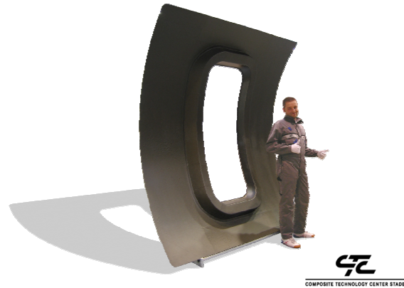
Fig.7: Assembly of the door surrounding structure on the prepreg shell (left), finished door cut-out with reinforcement made in CPI technology (right)
