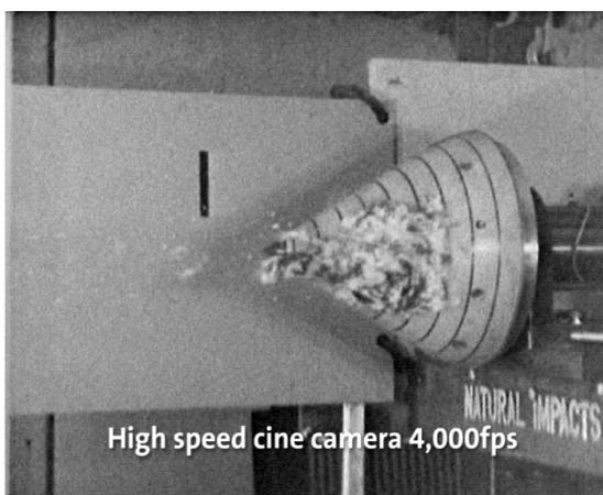
FIG 10. Nose cone during bird strike
