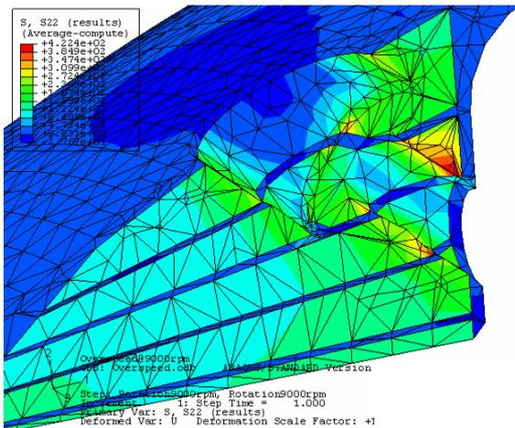
FIG 9. Hoop stress distribution in the highest loaded flange region
