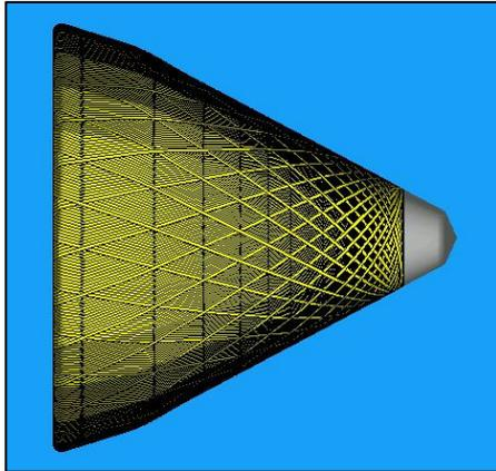
FIG 5. Simulated filament winding pattern
