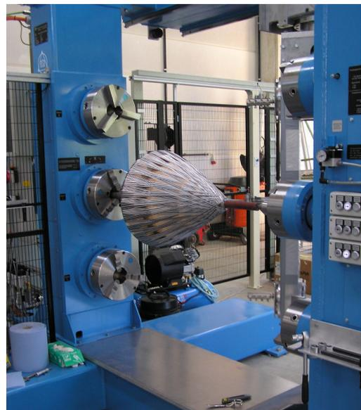
FIG 4. Automated filament winding
