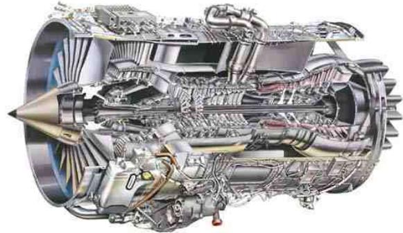
FIG 1. Section through BR715 engine
