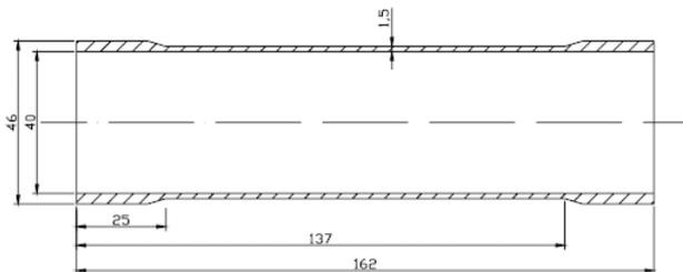
FIG 6. Tubular specimen for laminate test
