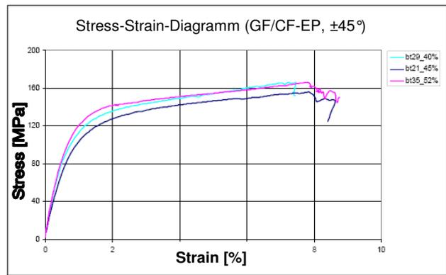
FIG 7. Stress-strain-curve in dependency of the fibre volume fraction
