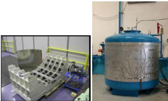
FIG 40. clamping tool design (Dassault Aviation) – left P180 fuselage barrel test – right
