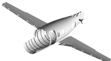
FIG 3. parts assembled by FSW technology on Eclipse 500 aircraft
