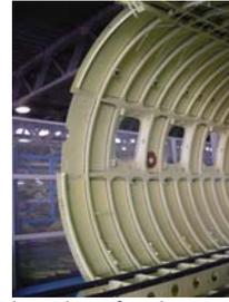
FIG 4. stringerless fuselage architecture on P180 business aircraft
