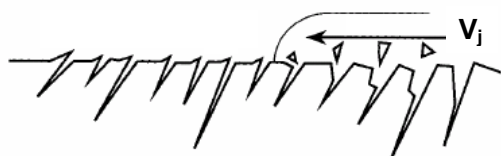
Fig. 4: Damage effects of lateral jetting; left hand side damaged by Rayleigh wave only; as lateral jetting crosses surface it tears off asperities it collides with [10].
