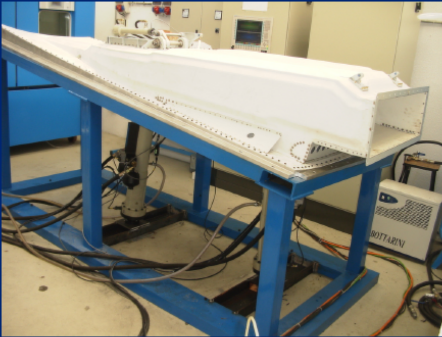
Mechanism fatigue test. AGU NACA Airbus A380
