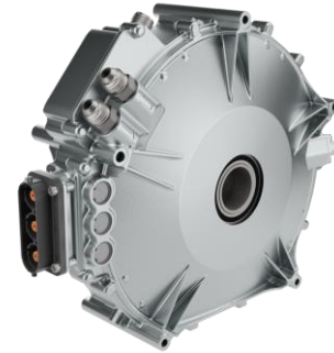
Evolito D500 1x3 Liquid cooled axial flux 350kW 9000rpm 12kW/kg peak
