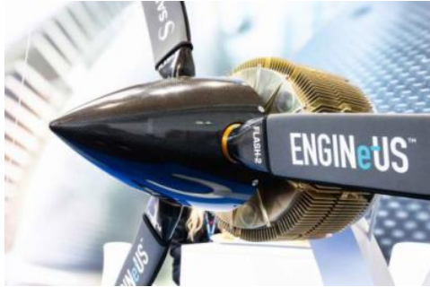
Safran ENGINEUS 100 Air cooled PM radial flux 125kW 3500rpm 5kW/kg peak, 3.5kW/kg continuous
