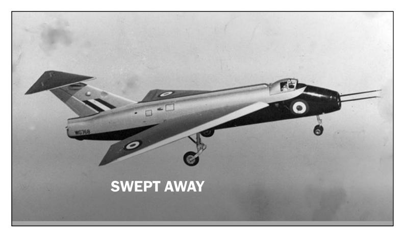
**Shorts SB5 research aircraft** to provide input for the design of the English Electric P.1 (prototype of the English Electric Lightning) by testing the low speed flight characteristics of various configurations of wing-sweep required for supersonic flight.
