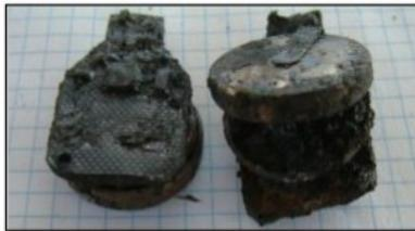
Lithium primary button sized flat cell batteries (watch style) with small circuit board
