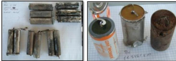
Additional battery pack remains [LH]/D-Cell size lithium primary batteries. Photo shows fire damaged and undamaged batteries [RH]
