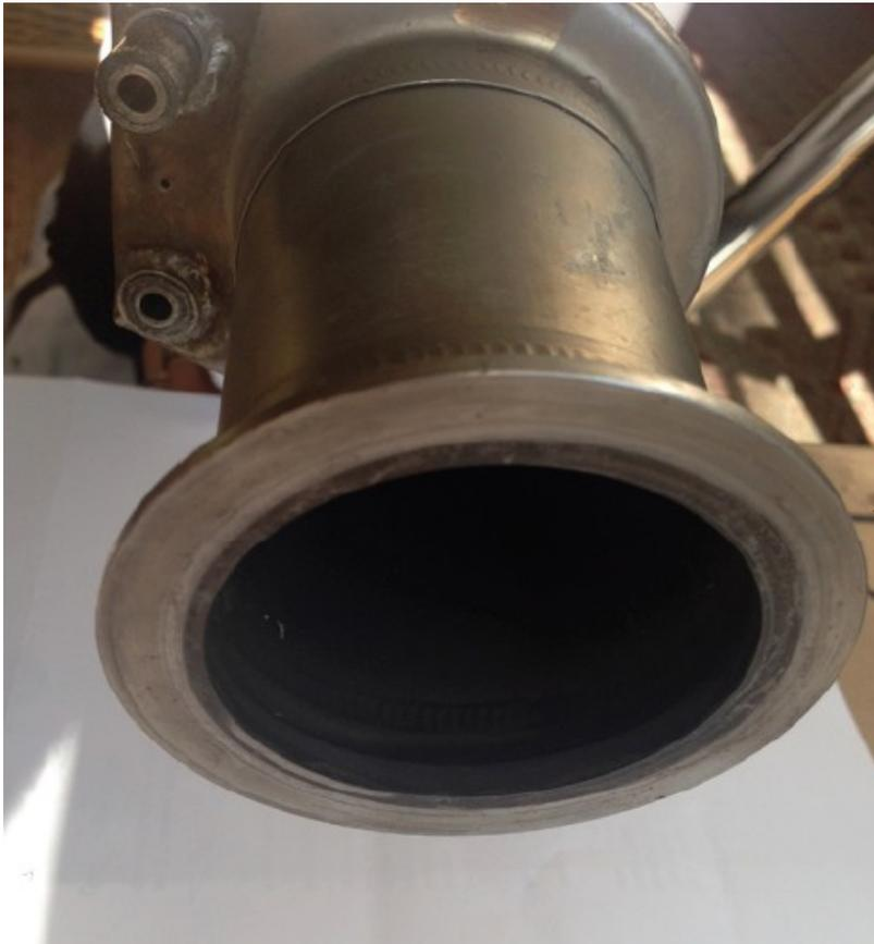
Visual inspection of a bleed air off-take port from a Boeing 737. The interior is black from oil contamination. (GCAQE 2017)
