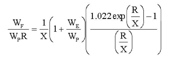
W<sub>F</sub>=Fuel Weight W<sub>P</sub>=Payload W<sub>E</sub>=Aircraft Weight-Empty R=Range  $X = H\eta L/D$
