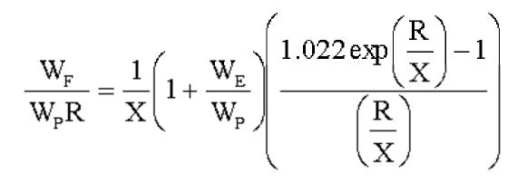
W<sub>F</sub>=Fuel Weight W<sub>P</sub>=Payload W<sub>E</sub>=Aircraft Weight-Empty R=Range
