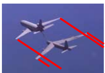
Fig. 17 FIXED OR VARIABLE SWEEP OBLIQUE WING CONFIGURATIONS
