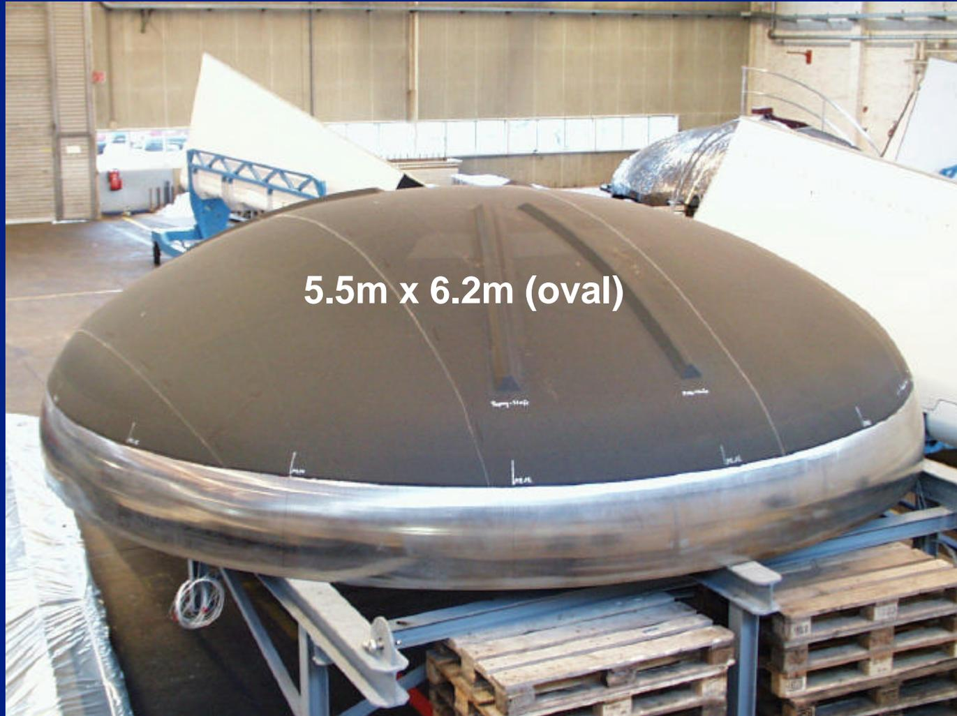
**A380 Rear Pressure Bulkhead: Resin Film Infusion (RFI)
