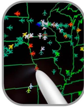
Figure 36. Air Traffic Control & a day plan at NATS, Prestwick (19 Jan 2015), Oceana Traffic in Tubes 60nm apart, Longitudinal Separation 10 mins to allow for different speeds and heights
