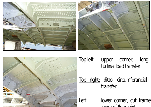
FIG 13. Structural surrounding of a passenger door
