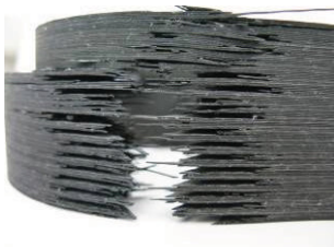
FIGURE 11. Tension failure of QI specimen: sub-groups of 4 plies (left) disrupted subsection (right)
