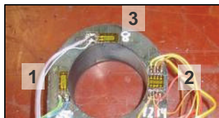
FIGURE 6. Distribution of strain gauges including the numbering of the strain gauge positions
