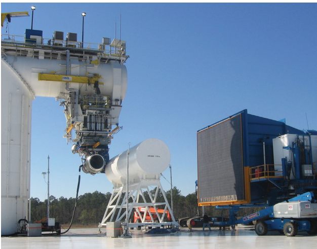
Figure 1 Engine certification testing with crosswind blower and fuselage simulator using the Rolls-Royce test facility at Stennis Space Center Mississippi.
