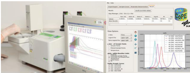
FIGURE 14: Measurement of reaction kinetics of the resin (10)
