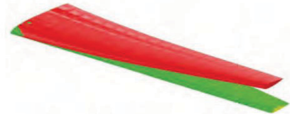
FIGURE 2: Global and local Displacement of a Wing (6)
