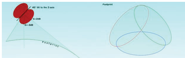
Figure 2: Antenna footprint for dipole tilted 45 degrees relative to z-axis
