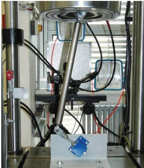
Fig. 14: Secondary strut test set-up
