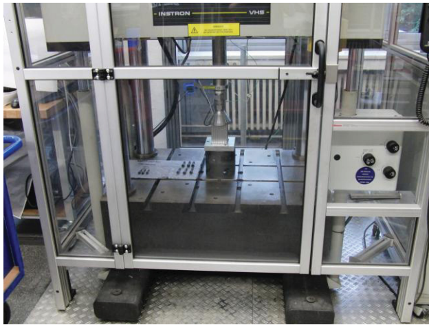
Fig. 10: Instron VHS 65/25 high strain rate testing machine with the test set-up
