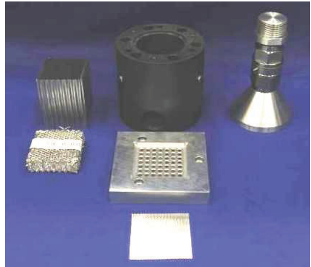
Fig. 7: Samples (left), lower compressing plate with air vents (middle) and upper compressing plate with a force sensor (right)
