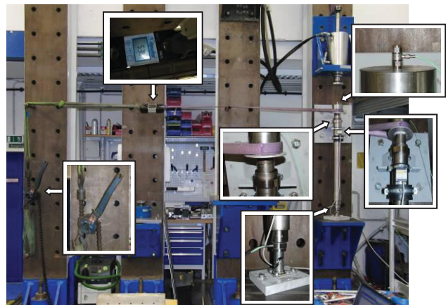
Fig. 16: Setup for bearing friction tests
