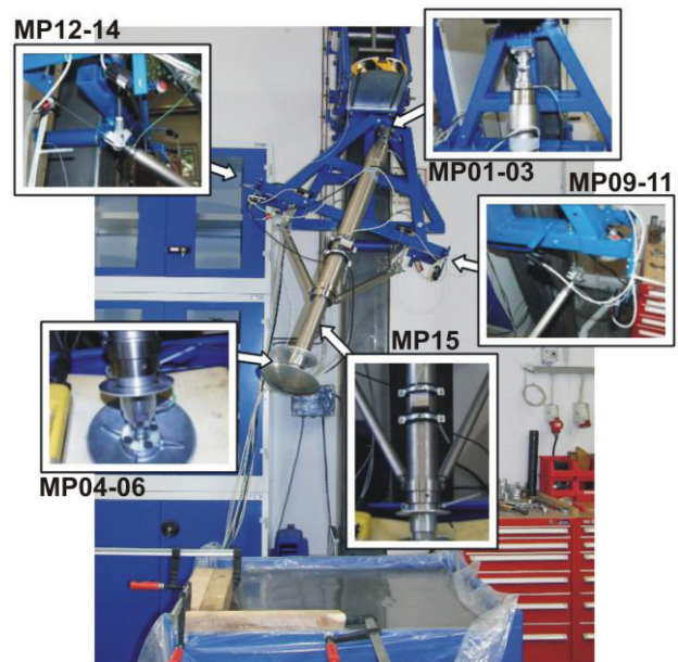
Fig. 23: Test setup of Cantilever Leg drop test
