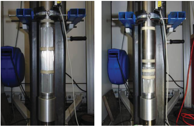
Fig. 18: Primary shock absorber before and after test
