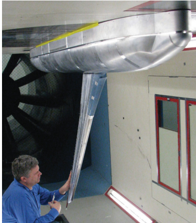
Figure 1: Industrial half-model in Bremen Low Speed Wind Tunnel (BLSWT) [1]
