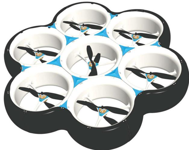
FIG 2. CellDrone made from seven cells
