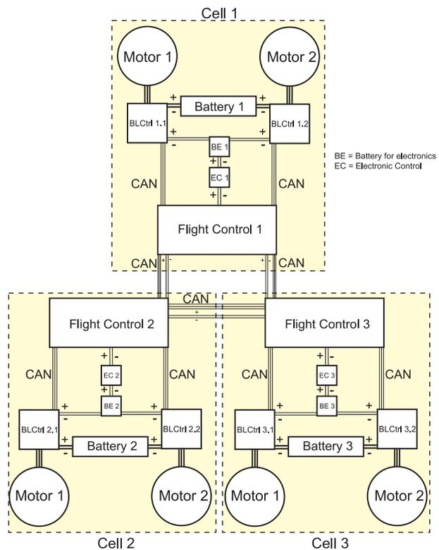
FIG 14. Electronic schematic of a CellDrone (three cells)
