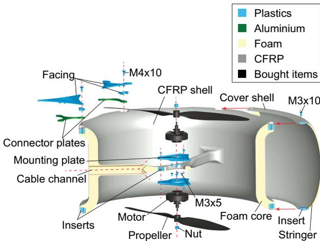
FIG 13. Cross-section of one cell
