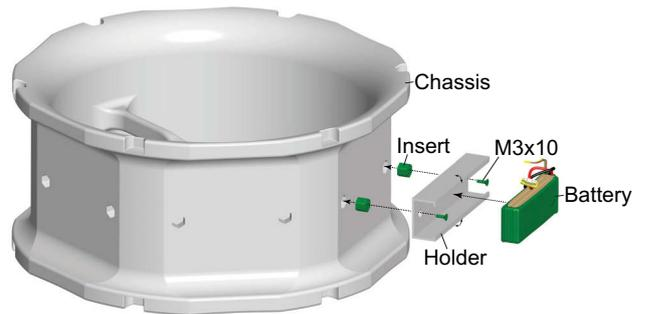
FIG 4. Connection between battery and airframe
