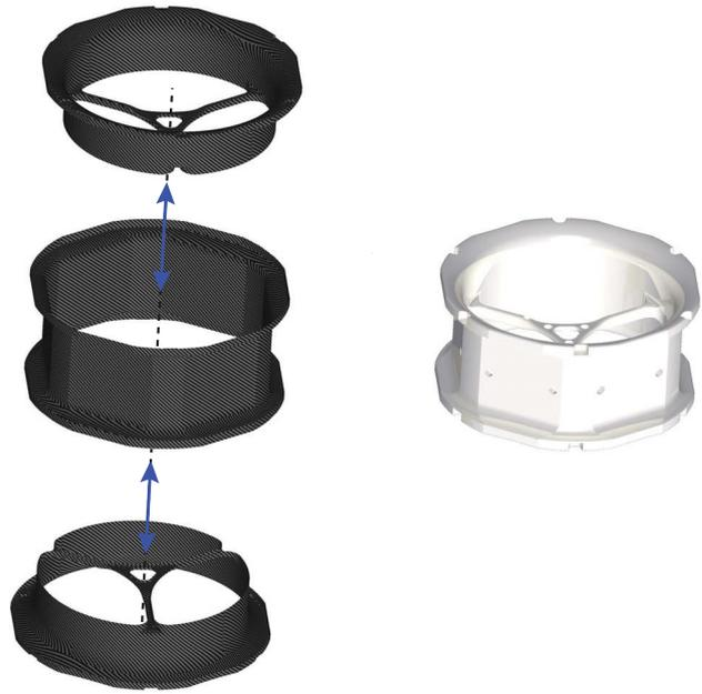
FIG 9. CFRP shell around foam core
