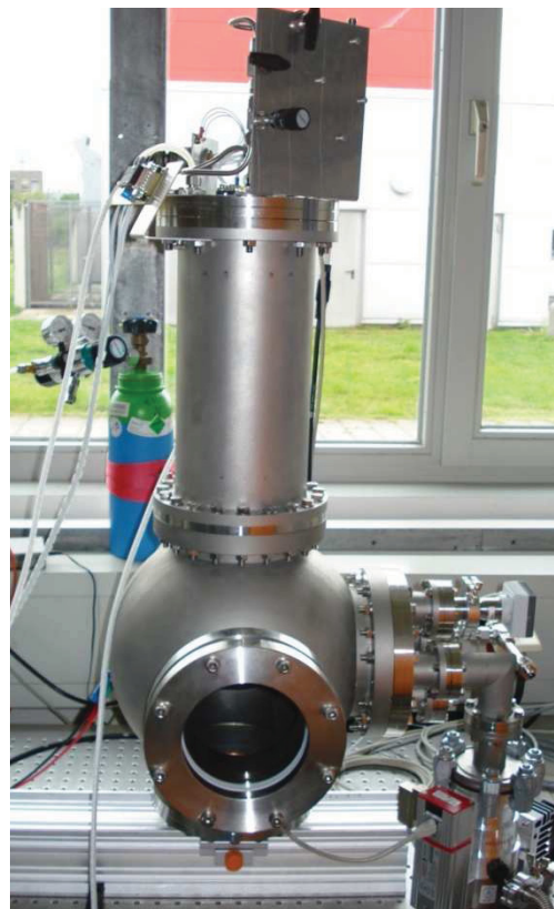
FIGURE 2. Vacuum chamber with mass flow controller and turbo-molecular vacuum pump
