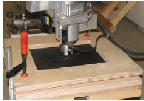
FIG. 20. Impact testing of sandwich CAI-specimens
