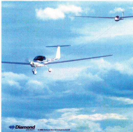
Figure 2.4: Diamond HK36 Super Dimona towing a glider, picture with kind permission of Diamond Aircraft [9]
