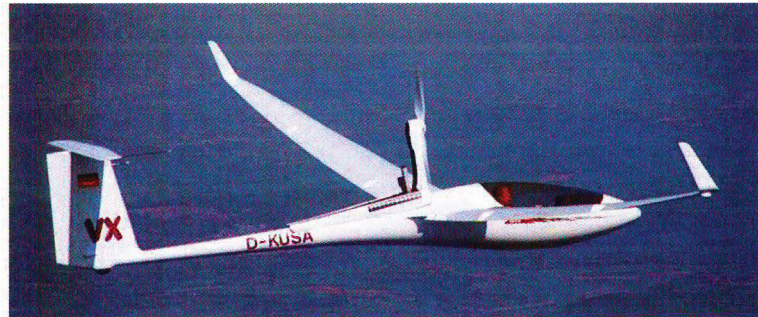
Figure 2.5: Alexander Schleicher ASH 31 Mi high performance self-launching glider with extended propeller, picture with kind permission of Alexander Schleicher Flugzeugbau [11]
