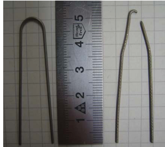
FIGURE 12. Elongation and fracture of Ti loop without welding: before (left) and after tensile test (right)
