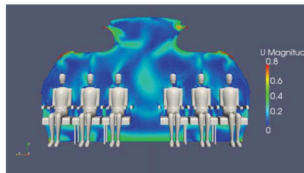
Fig. 10: Instantaneous velocity magnitude distribution obtained in one segment, with radiation modelling at t=42s
