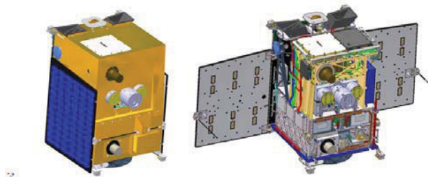
FIG. 4. TET-1 satellite: launch configuration (left), deployed w/o MLI (right)
