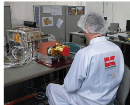
FIG.6. Payload N15 (Infrared Camera) acceptance test
