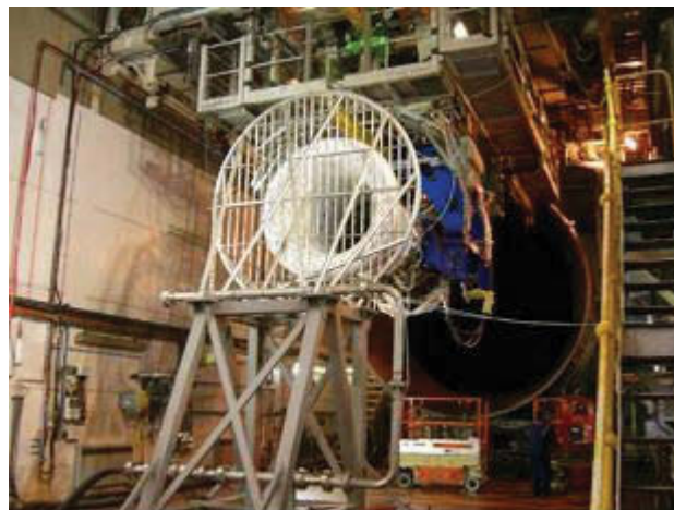
FIG. 11. Water spray grid in position during testing
