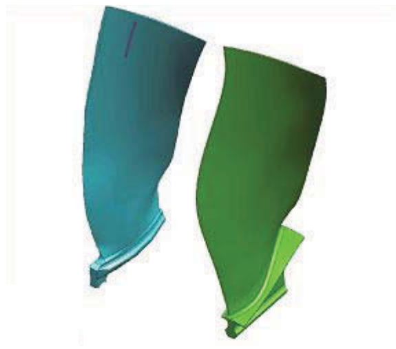
FIG. 2. BR710 fan blade (left) vs BR725 (right)
