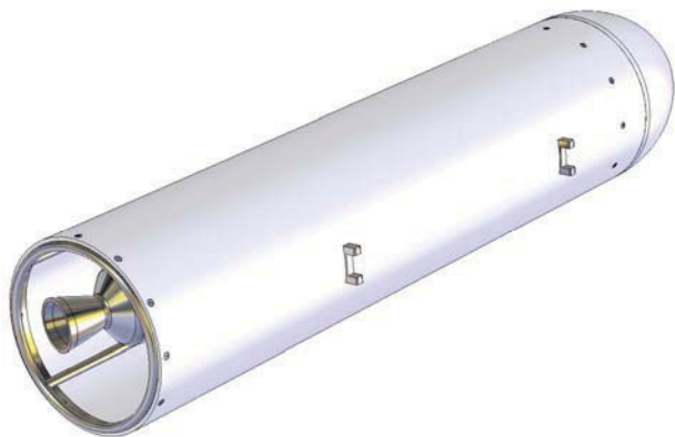
Figure 16. Concept of a reusable launch GRM for drones and UAVs
