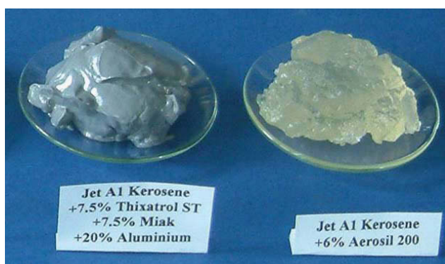
Figure 1. Examples of gelled fuels
