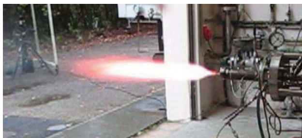
Figure 10. Test run of a gel model rocket combustor at DLR at Lampoldshausen
