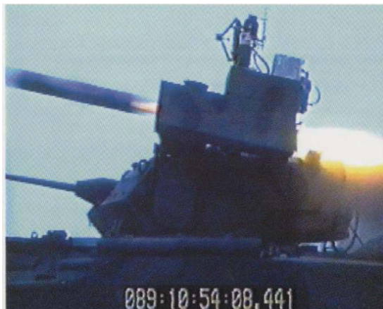
Figure 12. First launch of a gel missile [2]
