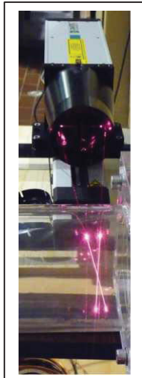
Fig A.1: Laser beam crossing at a point inside the straight pipe.
