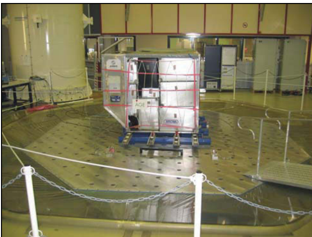
Figure 1: ULD Shaker Test campaign has been performed on a six-axis shaker table at ESTEC, Noordwijk (NL).
