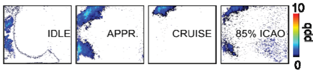
Fig. 6: Spatially resolved, time-averaged soot distributions for defined ICAO conditions.
